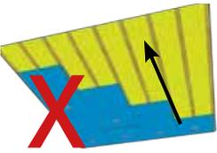
Keine Montage parallel zur Unterkonstruktion |
